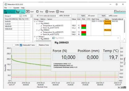
In the **Log view**, the user sets the logging details, the evaluation points - time for t0 and F0, and starts the test.
