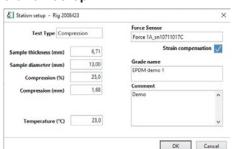
In the **Station Setup** window, the user sets the type of test (compression or tension) and the test piece dimensions.
