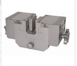
With a main shaft, both jaws are moved symmetrically at the same time and pre-tension the test specimen. If necessary, the connection can be disengaged to enable asymmetrical clamping, e.g. for shear tests.
