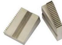
SP243-BV -V-jaws • For all kinds of round samples • Hardened steel 58 HRC • Tooth pitch 1.2 mm
