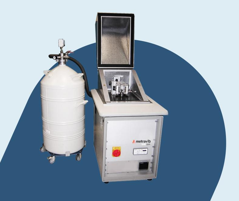
Such a test requires only a few minutes, while traditional approach using DMA low frequency test on several temperature stages, requires a few hours test and a calculation through WLF law.
